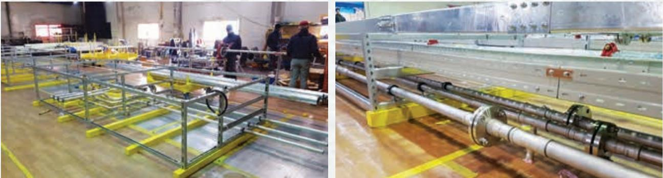
***DfMA – Pre-connection between Mechanical, electrical and plumbing service modules***
